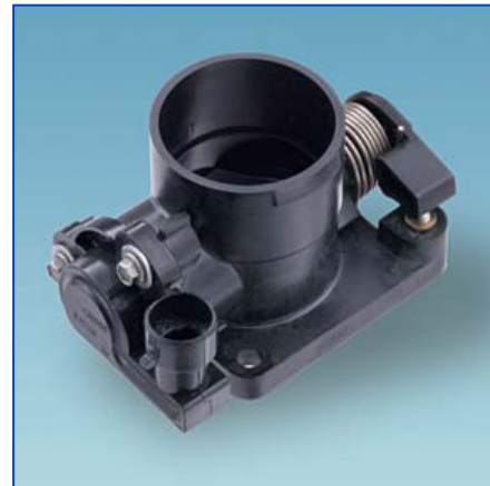
Delphi Composite Mechanical Throttle Body
