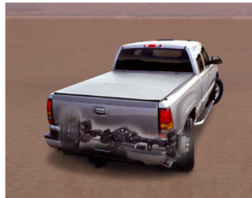
Delphi Quadrasteer™ Four Wheel Steering
